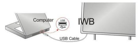
2.2 Connect the other end of the USB cable to the USB port on the computer.
